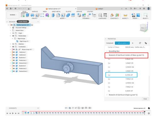
Note the value lyy (because the part rotates around the Y axis).
